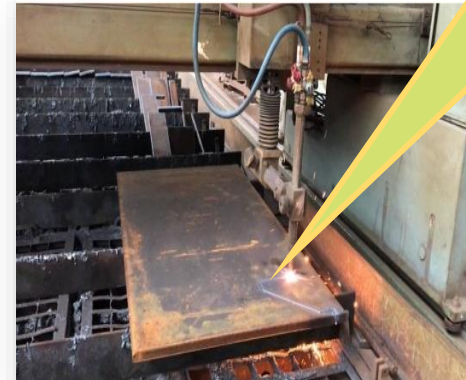
Manual Gas cutting using CBG with existing Oxy-fuel torch with no modification for manual cutting of carbon steel plates ranging from 10 to 25 mm sizes at Wagon component shop.
