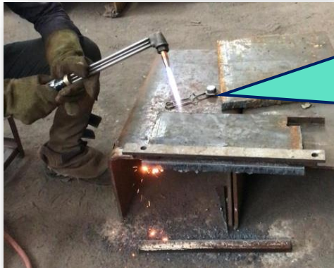
Manual Gas cutting using CBG with existing Oxy-fuel torch with no modification for manual cutting of carbon steel plates ranging from 10 to 25 mm sizes at Wagon component shop.
